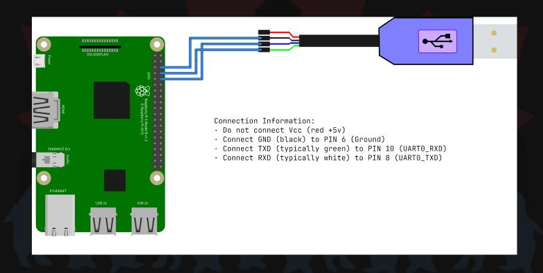
Connecting the red wire (Vcc) will attempt to power the Pi from this 5v port and we are not doing that here.
